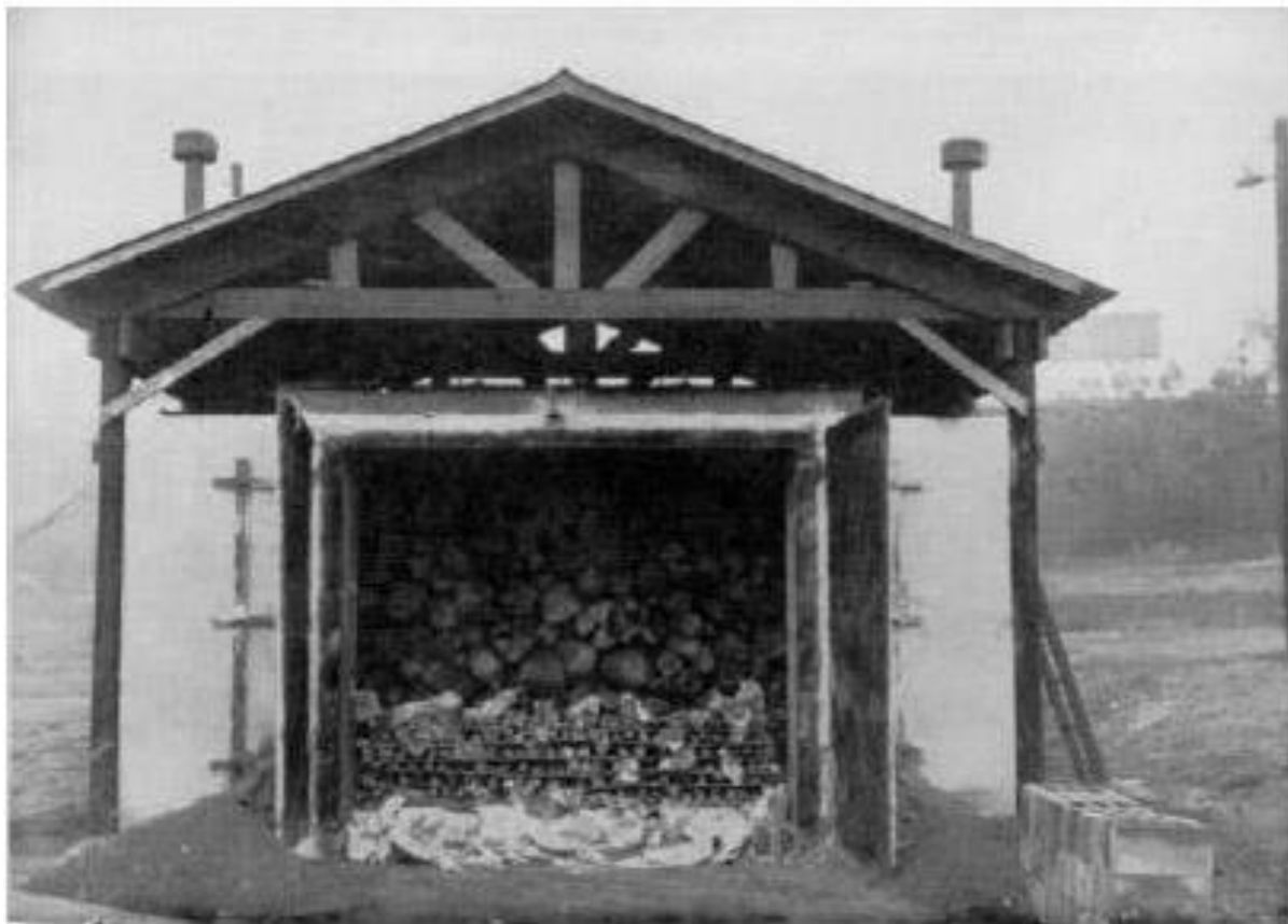
-Fuel stacked for ignition of a kiln in charge of seasoned wood.
